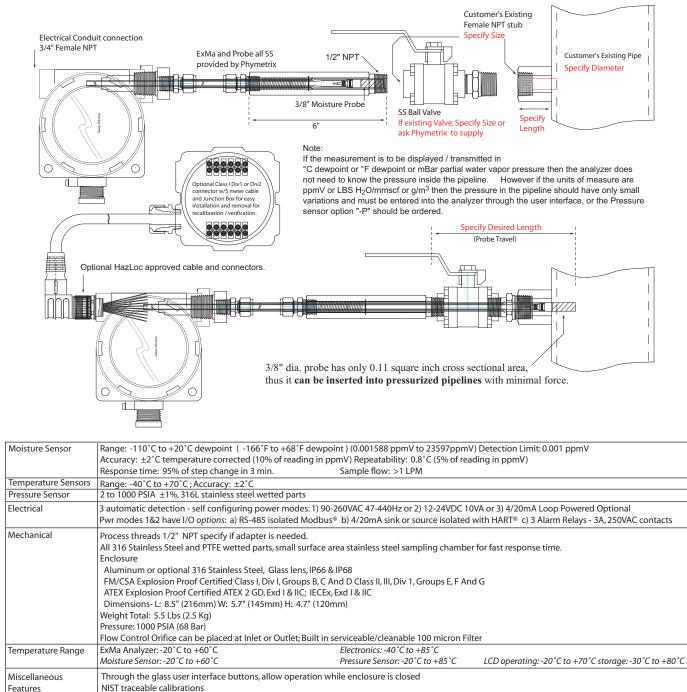
Units of measure: "C & "F dewpoint, ppmV, ppmV,  $\mu$ B H<sub>2</sub>O vapor pressure, grams of H<sub>2</sub>O / m<sup>3</sup> and Lbs H<sub>2</sub>O /10<sup>6</sup> standard cubic feet in Natural Gas Virtual Analyzer PC software for training and evaluation, allows the user to experience the exact interface on their own PC with voice explanations Optional Modbus® has ASCII and RTU modes
